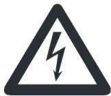
A lightening flash as an arrow symbol in a triangle indicates the presence of dangerous electrical voltage. Instructions marked with this symbol must be strictly followed. Otherwise, there is a risk of dangerous electrical shock to you or a third party, a short circuit or a fire. We recommend that all work is only carried out by qualified personnel.
